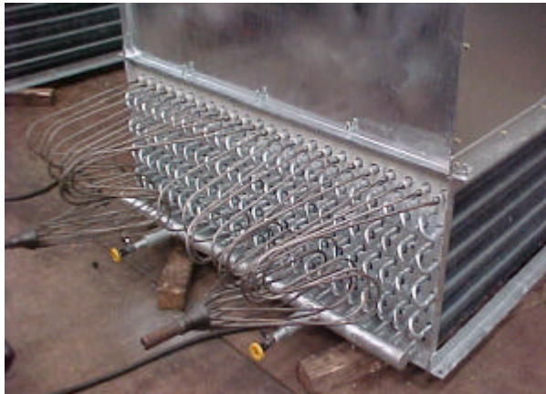
Figure 8 – Ammonia air-cooling evaporator Showing two liquid distributors and suction headers.
